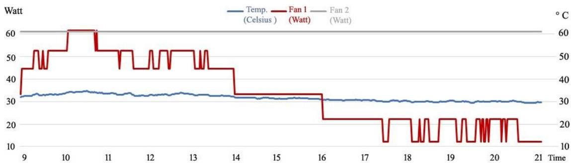
**Figure 11. The temperature and power consumption of the fans**
