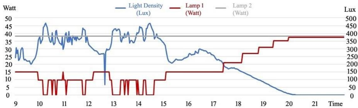
**Figure 10. The light density and power consumption of the lamps**
