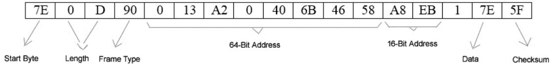
**Figure 2. A sample data frame in API mode**
