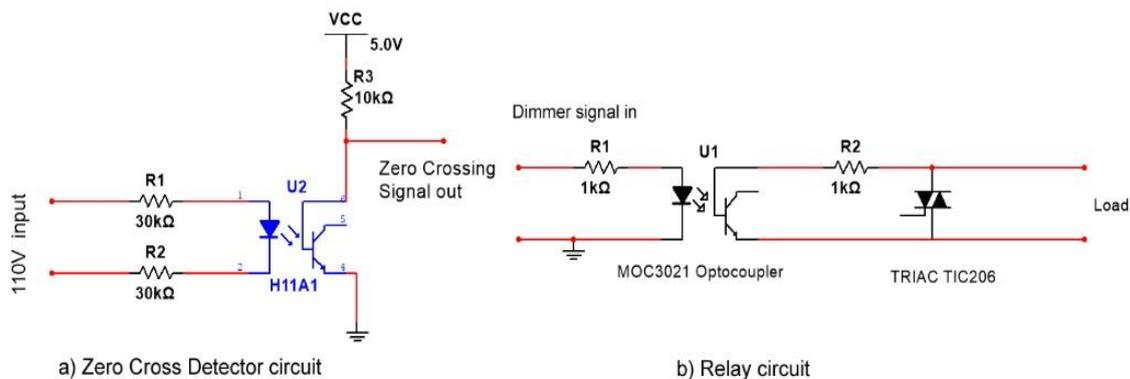
Figure 7. The zero-cross detector and solid-state relay
