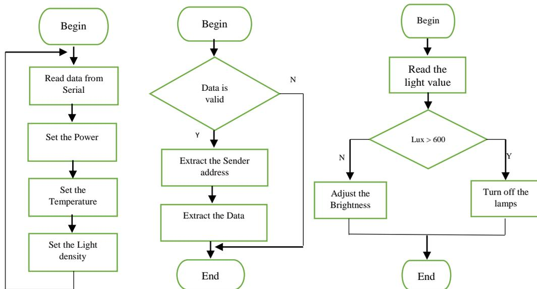
a) The Main function      b) Receiving data from XBee      c) Adjusting the light density
